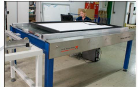
With the innovative J. v. G. LED 12.20 Flasher each module is tested not just once, but five times in one go. From this an average is derived which in turn will ensure that the results are more accurate. And that means, later for the dimensioning all wiring connections can be done much more precisely. The advantage is that the LED variant requires less time to determine these five test results than a common flasher for only one test cycle.
